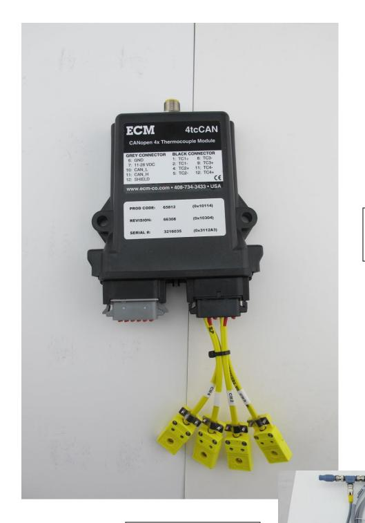
145mm x 120mm x 60mm IP67 Mini K-Type Connections
