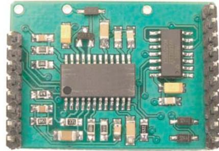
The AFM9 is a universal wideband lambda sensor controller that adds lambda, air-fuel ratio, and oxygen-measuring capability to your company's engine controller. Just plug or solder the compact AFM9 to your controller's circuit board and wideband sensor information is available through an SPI interface and an analog signal.
