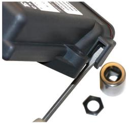
3. Slide the PCB out. Install a jumper on JP4.
