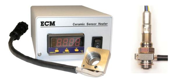
The ceramic sensor heater kit controls the mount temperature of a ceramic exhaust sensor. By doing this, the effects of an exhaust sensor's sensitivity to changes in mounting boss temperature (i.e. drift due to changes in exhaust pipe temperature) can be reduced. The NOx sensor used with the NOx 5210 analyzer and the NOxCAN module can especially benefit from this kit.
