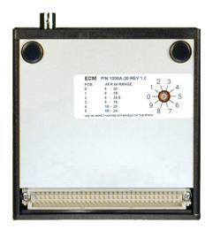
4. Plug the DJET1000 adapter module into the top of the stack. Make sure the pins in the connector engage properly and push it in straight.
