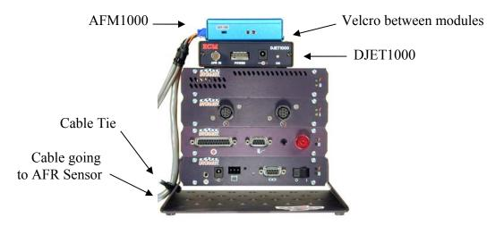
7. Plug the power connector on the wiring harness into the "POWER" socket on the DJET1000 adapter. Plug the black plug on the harness into the 12 VDC power socket on the Dynojet CPU module (the one with the little "+" sign in the middle of its label). Plug the BNC connector on the harness into the "AFR IN" BNC connector on the DJET1000
