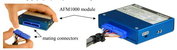
6. Sit the AFM1000 control module on top of the DJET1000 adapter module so that the AFM1000's ON-OFF switch is facing forward. Use the supplied velcro between the modules to hold them together. Use one of the supplied cable ties to tie the cable on the harness going to the AFR sensor to the base of the stack.
