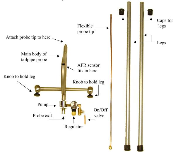
10. Assemble the tailpipe probe. You will need to get the proper fitting to match the one on your compressed air hose. The below pictures show important details of the assembly process.
