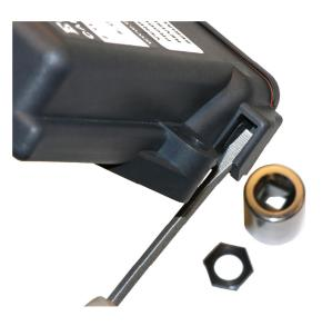
6. Slide the PCB out. Remove the jumper from JP4. You can hang it on one pin of JP4 when "off".
