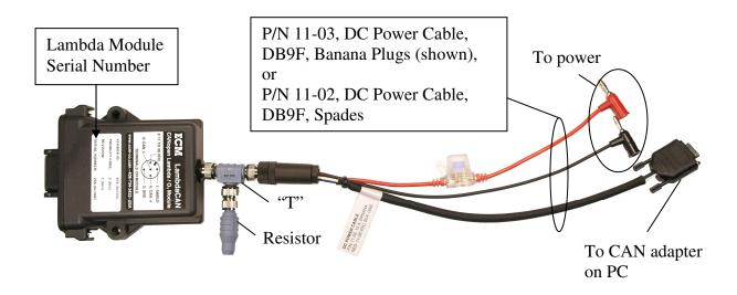
Figure B1: LambdaCAN Module prepared for Reprogramming
