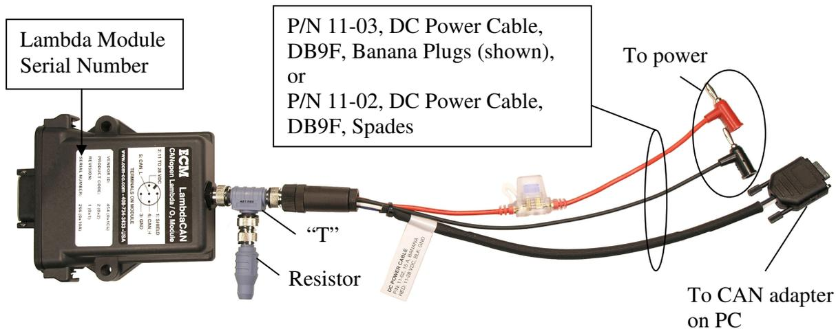
Figure B1: LambdaCAN Module prepared for Reprogramming
