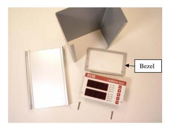
4. Sandwich the rackmount panel, <u>WITHOUT THE FRONT BEZEL</u>, between the front display and the aluminum base. Reinstall the two front screws.
