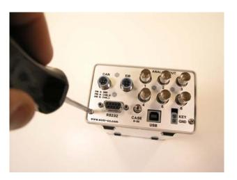
2. Slide the back panel and the main board out of the instrument. Do not separate the back panel from the main board.
