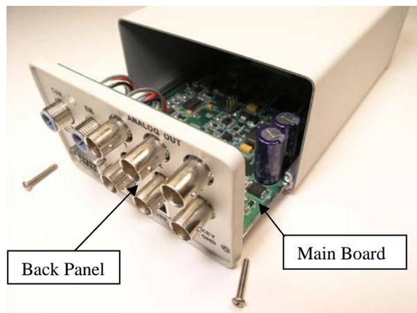
3. Remove the two screws on the front panel and separate the aluminum base, the top cover, the front display, and the bezel.
