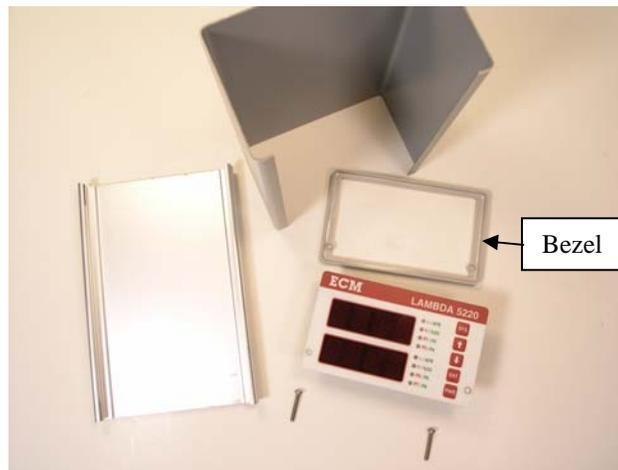
4. Sandwich the rackmount panel, WITHOUT THE FRONT BEZEL, between the front display and the aluminum base. Reinstall the two front screws. Do not overtighten the front screws or you will damage the front panel.
