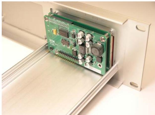
5. Install the top cover onto the aluminum base and slide it up to the front. Make sure the top cover fits into the correct grooves in the aluminum base.
