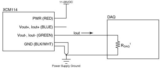
Current output mode, using **external** (**Ext**) power (i.e. Current Transmitter Type 4):
