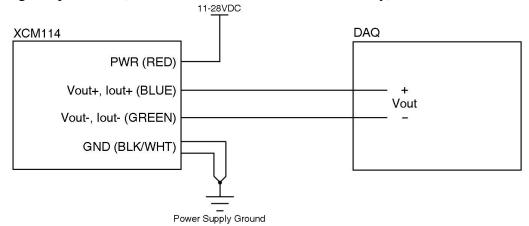
Current output mode, using **internal** (**Int**) power (i.e. Current Transmitter Type 3):
